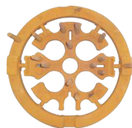
Cylinder head core Wall thickness - 12 mm
