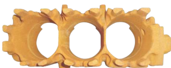
Cylinder block water jacket core Wall thickness - 4.0 mm
