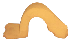
Core for impeller thickness - 20 mm
